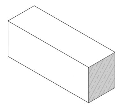
The process of working a column starts with a rectangular piece of stone, the dimensions of which match the required diameter and height of the finished piece. For this example the column is without entasis, that is, the sides of the column are parallel in elevation.
