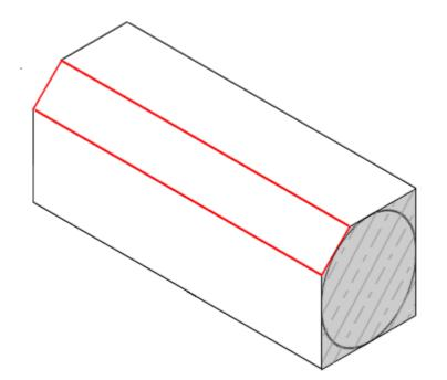
With the diameter of the column scribed, a series of chamfers are marked on the ends using a shift stock and joined together along the length of the stone. As shown in this picture, the initial chamfers are at 45° to the face edges and touch the scribed circle. Once scribed on, these four chamfers are worked along the length of the stone.
