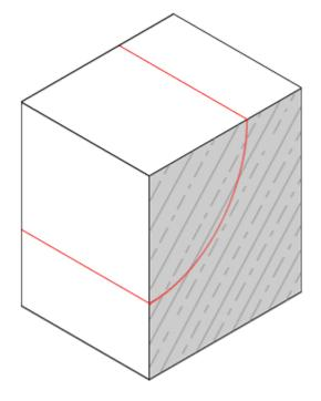
The process of working a cavetto begins by marking the template onto the parallel joints of the stone using a scriber. Templates for stone are traditionally made from zinc sheeting. With the template marked on, chamfers are worked from each side of the moulding towards the middle. This stage defines the deepest part of the mould, and like all stonework, using a straight edge ensures the mould remains true through the length of the stone with no high or low spots.
